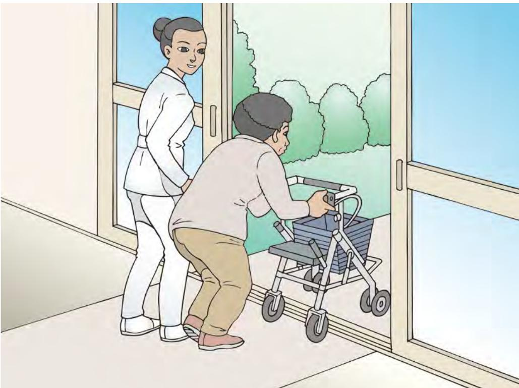
**Figure 1b.** Smooth movement and transport are secured by eliminating height differences in the entrance and corridors.
