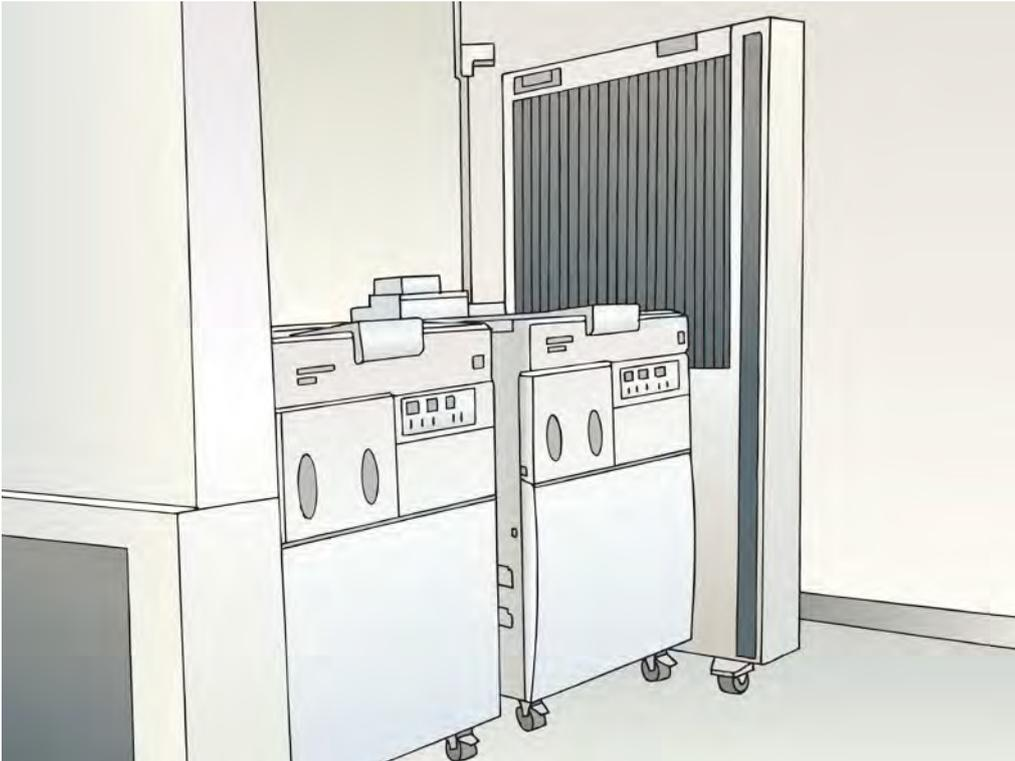
**Figure 33a.** Use local ventilation systems installed near a washing machine for endoscopes.
