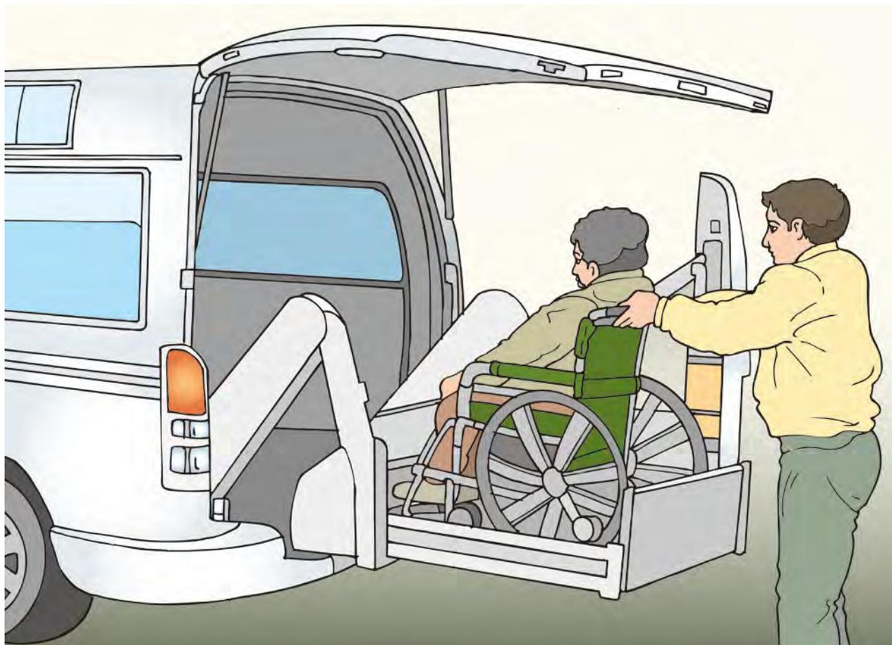
**Figure 18.** Service the vehicle's wheelchair lift as often as the manufacturer recommends. Record the maintenance in the vehicle logbooks.
