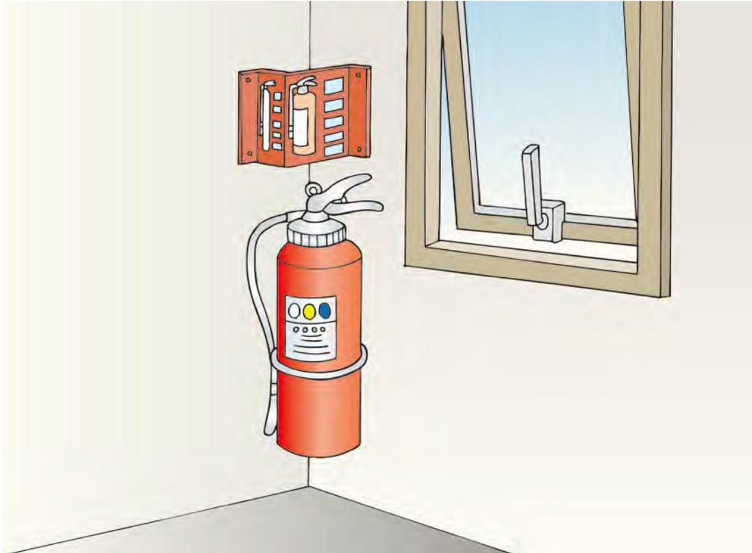
**Figure 52a.** Provide enough fire extinguishers at clearly designated places near work areas.
