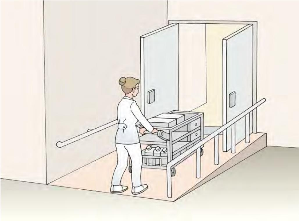
**Figure 1a.** Provide ramps with smooth surfaces to eliminate sudden height differences.
