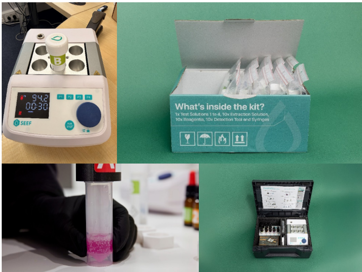
Top Left: Incubator With Sample. Top Right: Cr (VI) Sample Tube Kit. Bottom Left: Sample Positive. Bottom Right Cr (VI) Test Kit Case
